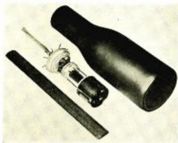
Cathode-ray tube for image projection. The interior ceramic structure is shown in detail.
