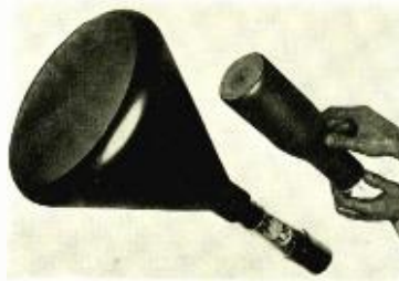
Comparison of the direct-viewing and projection type tubes; projector tube on the right.
